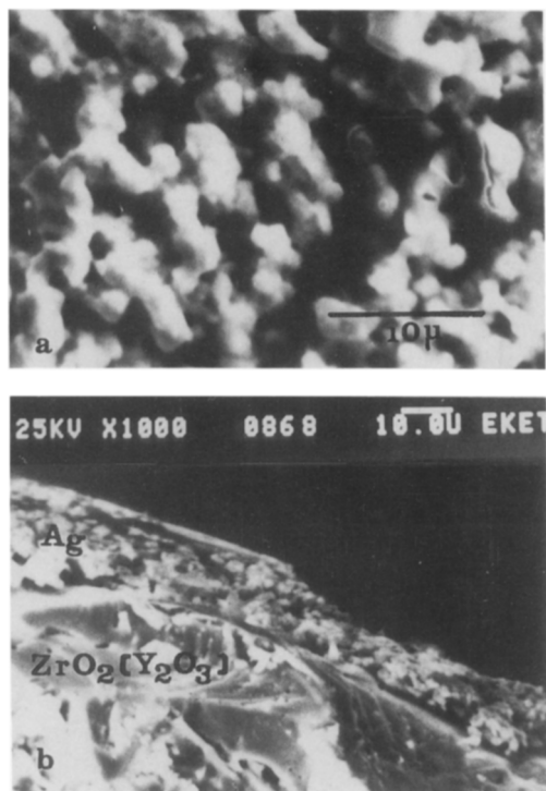
FIG. 3. Scanning electron micrographs of the top side of the porous Ag catalyst film (a) and of a section perpendicular to the Ag catalyst–yttria stabilized zirconia (YSZ) interface (b).
